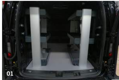
01 SORTIMO SR5 BASIC, RIGHT-HAND AND LEFT-HAND SIDE INC. FLOOR FOR VEHICLES WITH LONG WHEELBASE. Company-wide processes can be optimised even further by the SR5, and workflows become far more targeted and efficient. The shelving system has been designed to permit immediate access to the tools required and to allow loads to be stowed away clearly and in a well-structured manner. Drawers, cases and BOXXes as well as numerous accessories make the SR5 the perfect partner for every organisation in the skilled trade sector. The tried and tested ProSafe load securing system integrated in the van racking guarantees maximum safety for occupants and the load. Part Number: ZGB2SK061 673 (CA)
