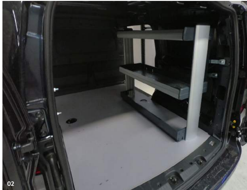
01 SORTIMO SR5 BASIC, RIGHT-HAND AND LEFT-HAND SIDE INC. FLOOR FOR VEHICLES WITH LONG WHEELBASE. Company-wide processes can be optimised even further by the SR5, and workflows become far more targeted and efficient. The shelving system has been designed to permit immediate access to the tools required and to allow loads to be stowed away clearly and in a well-structured manner. Drawers, cases and BOXXes as well as numerous accessories make the SR5 the perfect partner for every organisation in the skilled trade sector. The tried and tested ProSafe load securing system integrated in the van racking guarantees maximum safety for occupants and the load. Part Number: ZGB2SK061 673 (CA)
