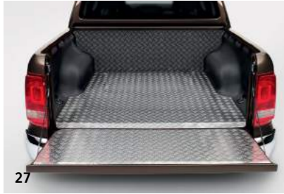
27 ALUMINIUM LOAD AREA LINER. Protects the load area and is fitted to the load floor, front wall and rear tailboard. The wheel arches and side walls are protected with contoured plastic. Part Number: 2H7061164J (AM)
